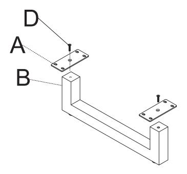
Use Screw (E) to connect the U Shape Base (B) and the Bracket (A) to the bottom of the Pedestal.
